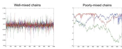
Monitor convergence by plotting samples from multiple MH runs (chains)
